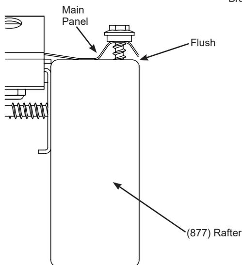
**DO NOT overtighten screws, could cause damage to roofing material**
