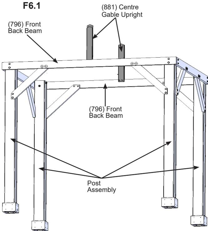
*Note: The Gable Uprights may have to be adjusted when roof is installed.*
