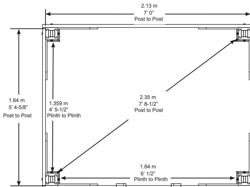
**Part Identification** ( Dimensions are approximate and are shown to assist in the identification of parts for assembly. Actual dimensions may be smaller or larger. )
