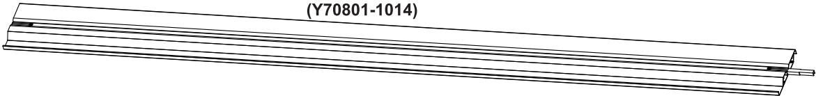
16pc. Louver Assembly B (2825mm ) (111-1/4")
