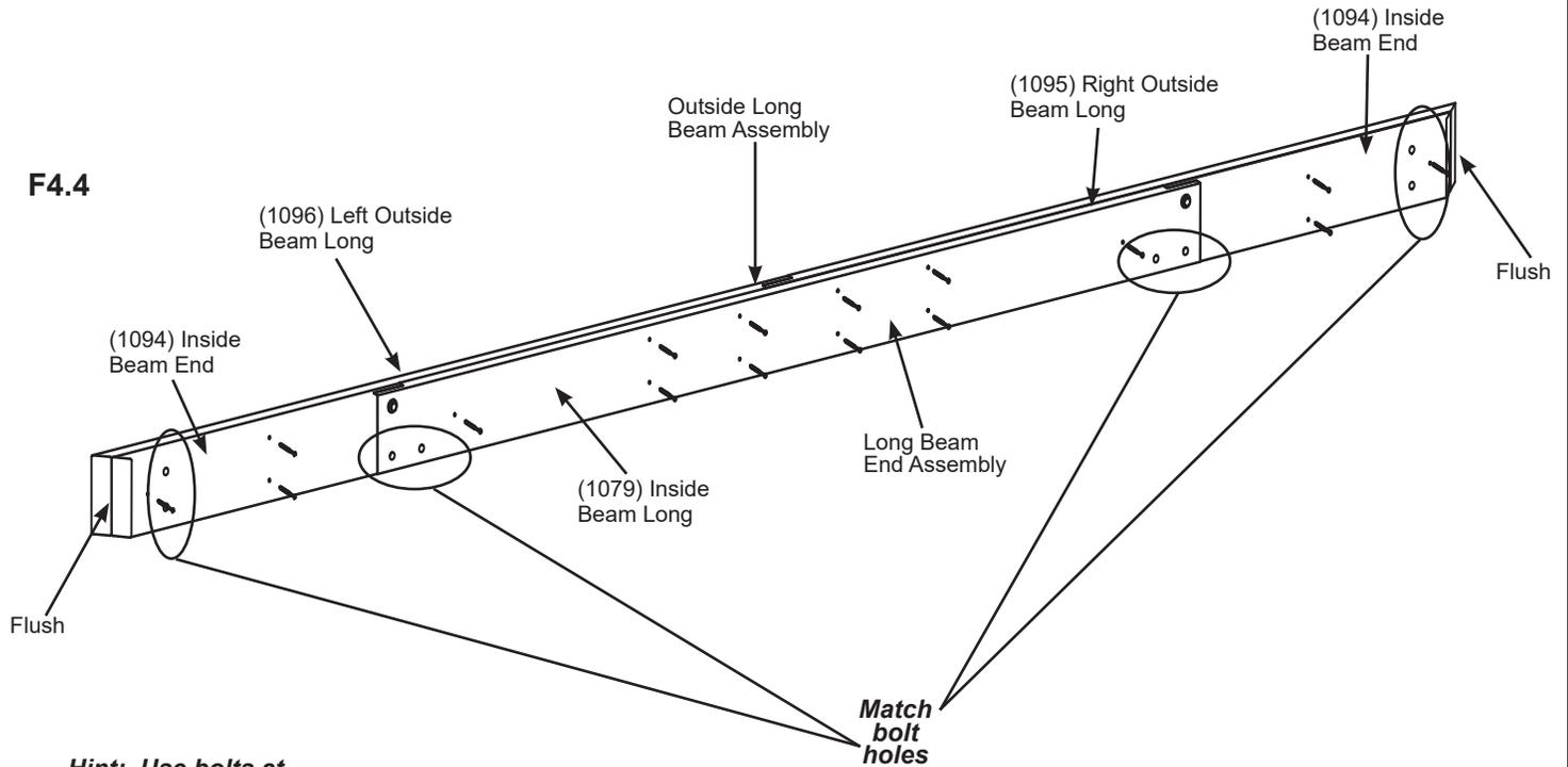
*Hint: Use bolts at both ends to line up bolt holes. Remove bolts once step is complete*
