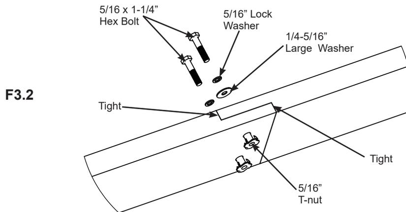
***Make sure bolt heads are on the outside of each Beam Assembly***
