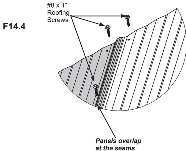
**DO NOT overtighten screws, could cause damage to roofing material**
