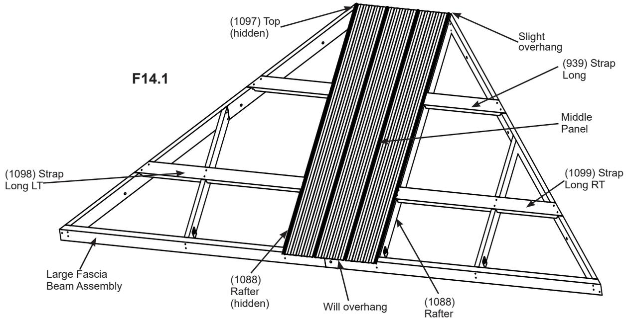
**DO NOT overtighten screws, could cause damage to roofing material**
